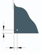
Through - fixing holes should be at least 1.5 times the outside diameter of the screw being used and should be positioned a minimum of 20mm from the edge of the panel.
