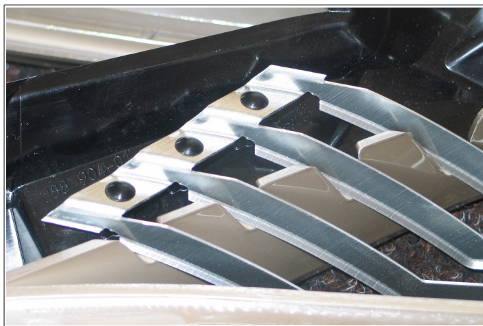
Jig 2×3 pins, distance of the pins 16 mm
